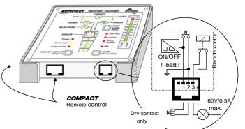
The Control Input is connected in parallel to the ON/OFF- push button. The COMPACT can be switched on or off through this input with an impulse button or an impulse contact.
